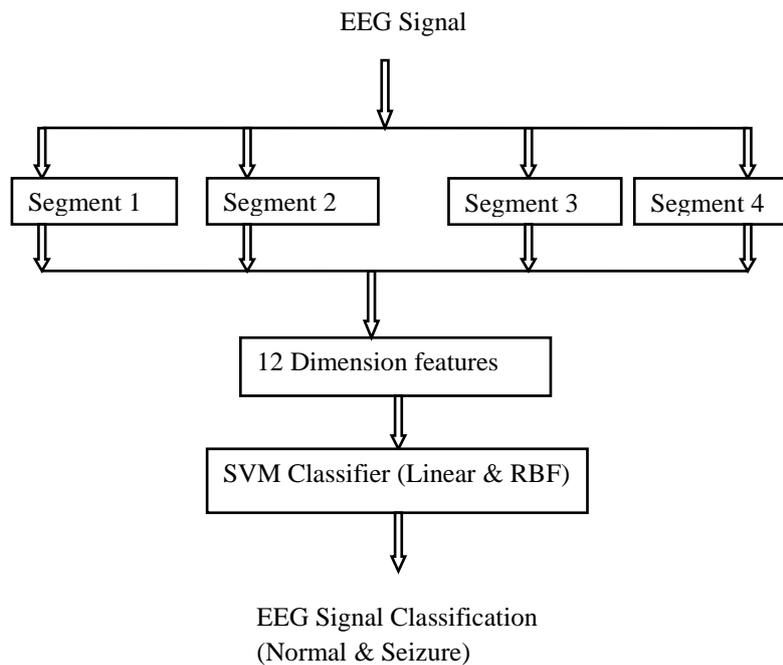
**Figure 1: Processing modules for EEG signal classification**
